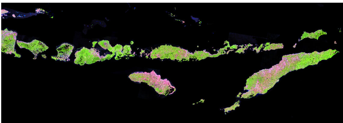
Figure 3.3. 2007 Landsat mosaic of Nusa Tenggara with bands 3,4,5 in BGR. The area shown is approximately 1500km by 500km. Black areas within the islands indicate areas of missing data due to cloud in 2007.
